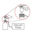
Attach the spin column to GREEN ADAPTOR fitted on the 45 mm neck bottle
